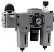
Ball Valve + Filter + Regulator + Lubricator Combinations, poly bowl 5 micron element, 116 psig (8 bar) regulator + gauge and wall mounting brackets
