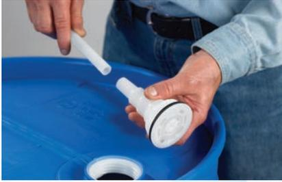
1 Fully press dip-tube into drum insert socket.
