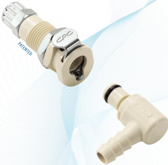
The 1/8" flow polypropylene PMC12 offers many of the same configuration options as the PMC. The polypropylene material adds greater chemical resistance and is gamma sterilizable. The PMC12 also mates to small diameter rigid tubing. Available with a 1/4-28 at bottom port and 1/4-28 UNF threads, these couplings eliminate the need to thread and re-thread common compression nuts each time a tubing connection is made.
