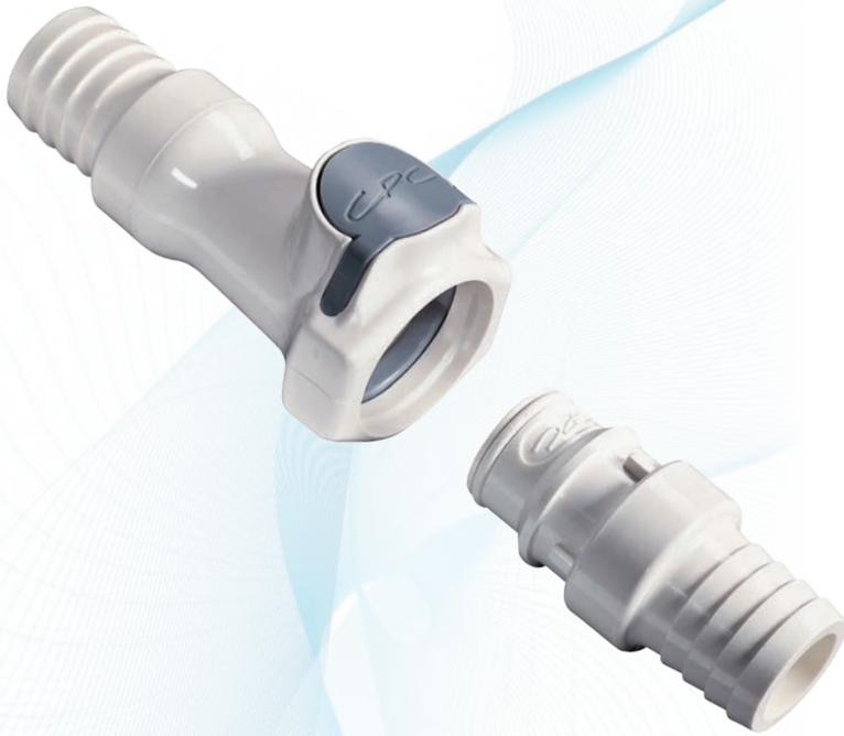
**FFC35 Series 1/2" flow couplings** feature double the flow of the HFC Series couplings. The FFC Series has a non-valved bore that increases flow and minimizes turbulence. The polysulfone material is able to withstand demanding applications and features physical strength, chemical resistance and autoclavability. An ergonomic design and a large, shrouded thumb latch pad produce a coupling that is easy to grip and simple to operate.
