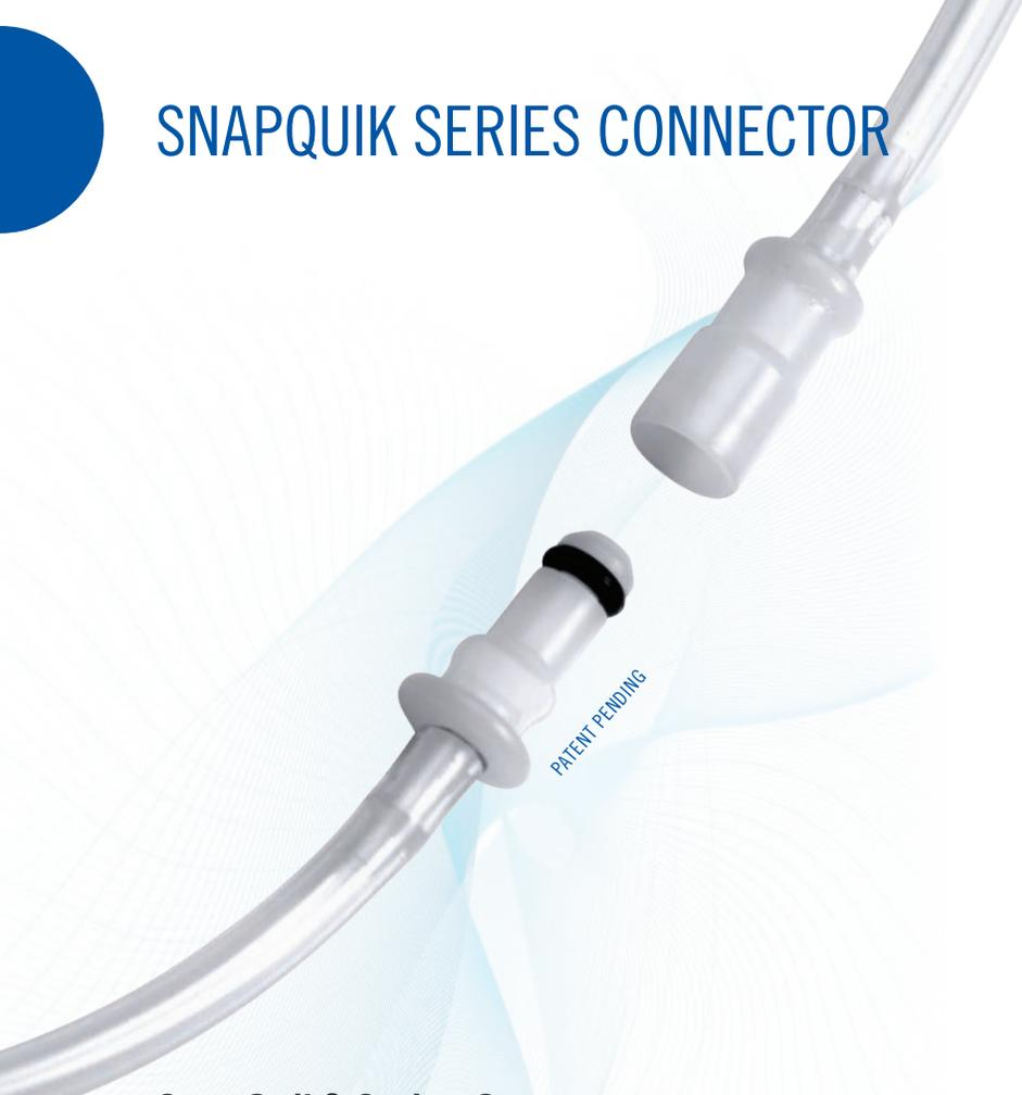
**SnapQuik® Series Connectors** are ideal for small bore applications. The compact design delivers high flow fluid transfer in a small profile. Featuring a unique internal latching mechanism that creates a smooth, streamlined exterior that is easy to clean and use. The user-friendly break away design of SnapQuik prevents misconnections with luers, protects equipment and ensures patient safety.
