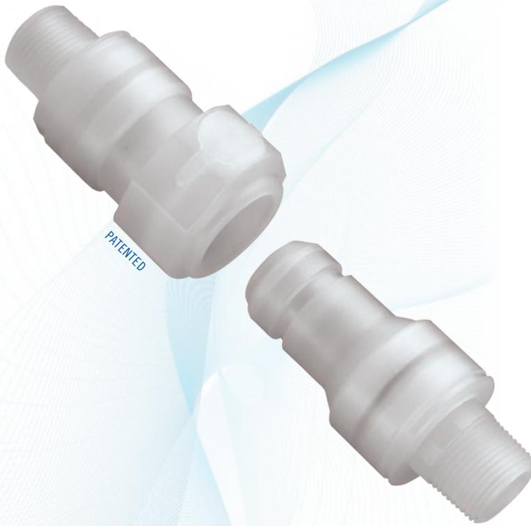
**The CQG06 Series** high purity couplings feature our patented pressure-balanced, non-spill design. Molded virgin polypropylene and a 100% springless flow path provide broad chemical resistance and exceptionally high flow capacity, allowing instant disconnects (and reconnects), even under pressure.
