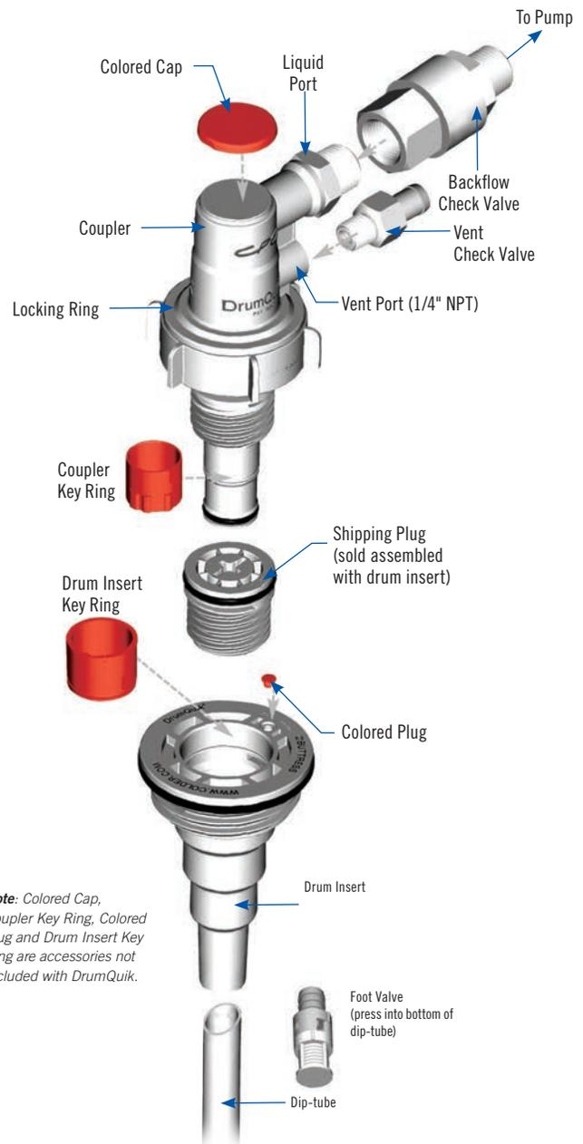
**Note:** Colored Cap, Coupler Key Ring, Colored Plug and Drum Insert Key Ring are accessories not included with DrumQuik.
