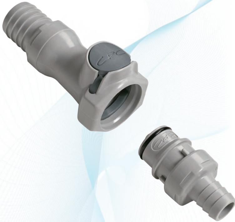
**HFC12 Series couplings** have flow comparable to many 1/2" couplings in a 3/8" body size. Compact and lightweight, HFC couplings replace bulky and heavy brass ball-and-sleeve couplings in a wide range of applications. An ergonomic design and a large, shrouded thumb latch pad produce a coupling that is easy to grip and simple to operate. An efficient valve design leads to high flow and low spillage.
