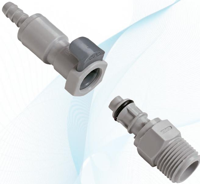
The **9/32" flow EFC12 Series couplings** feature a high efficiency valve design that provides a greater flow capability than any other coupling its size. Chemically resistant polypropylene material makes it ideal for harsh environments. The EFC12 Series adds a bulkhead panel mount option for tight seals against tank walls and drums.
