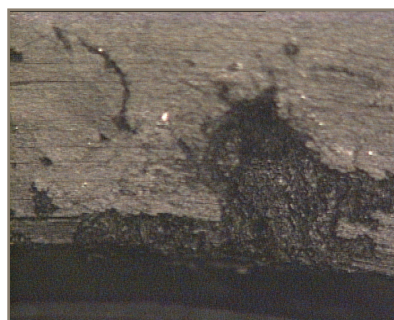
Pitting on filter end-cap
