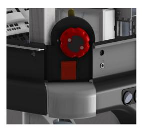
3 Turn off the power relays in the front-left corner of the robot. Make sure to turn them off starting with the inner-most relay.
